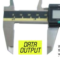
When this point is established, the distance from this position will always be displayed, the intelligent memory retains the 'origin point' even when powered off. Infinite response speed, large ICD feature.
