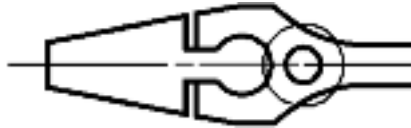
Tapered Jaw For Access Into Tight Spaces
