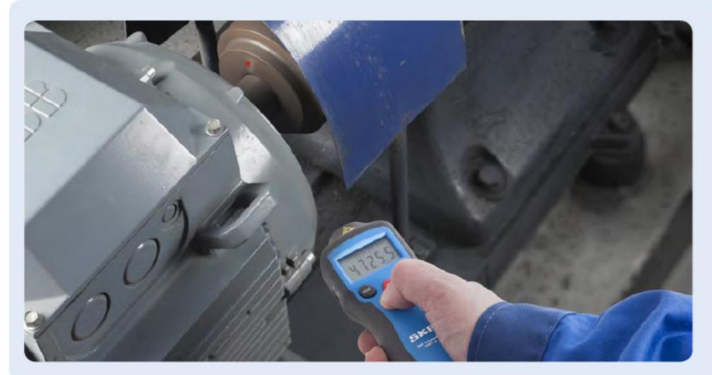
The laser optical system allows easy and quick measurements at a safe distance from rotating machinery.
